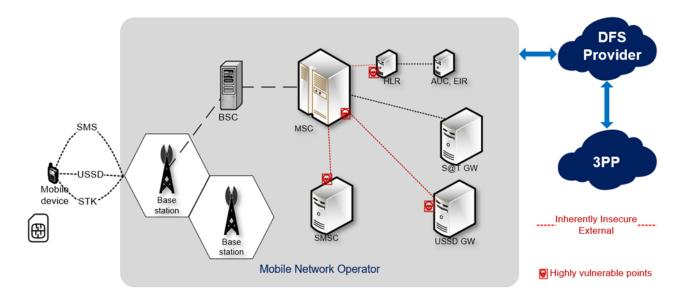
Figure 4 shows the various points at which the DFS data is captured within the ecosystem.
